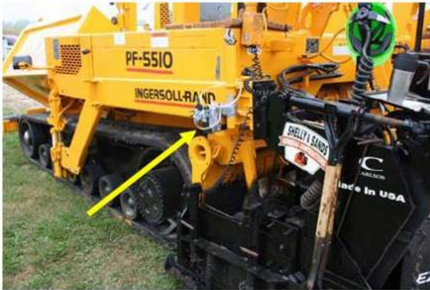
Sample Location 2 – Left Side Screed Discharge over Auger
