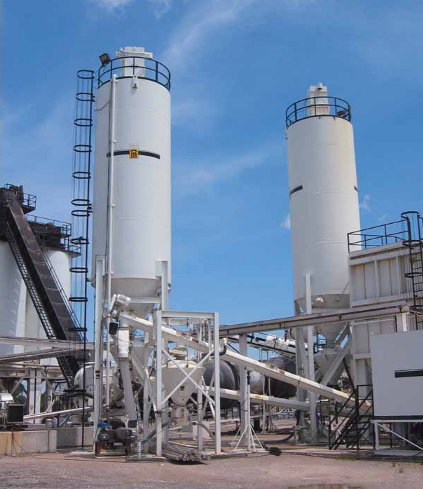
Pace's plant had minimal problems producing warm-mix asphalt for the paving project.
