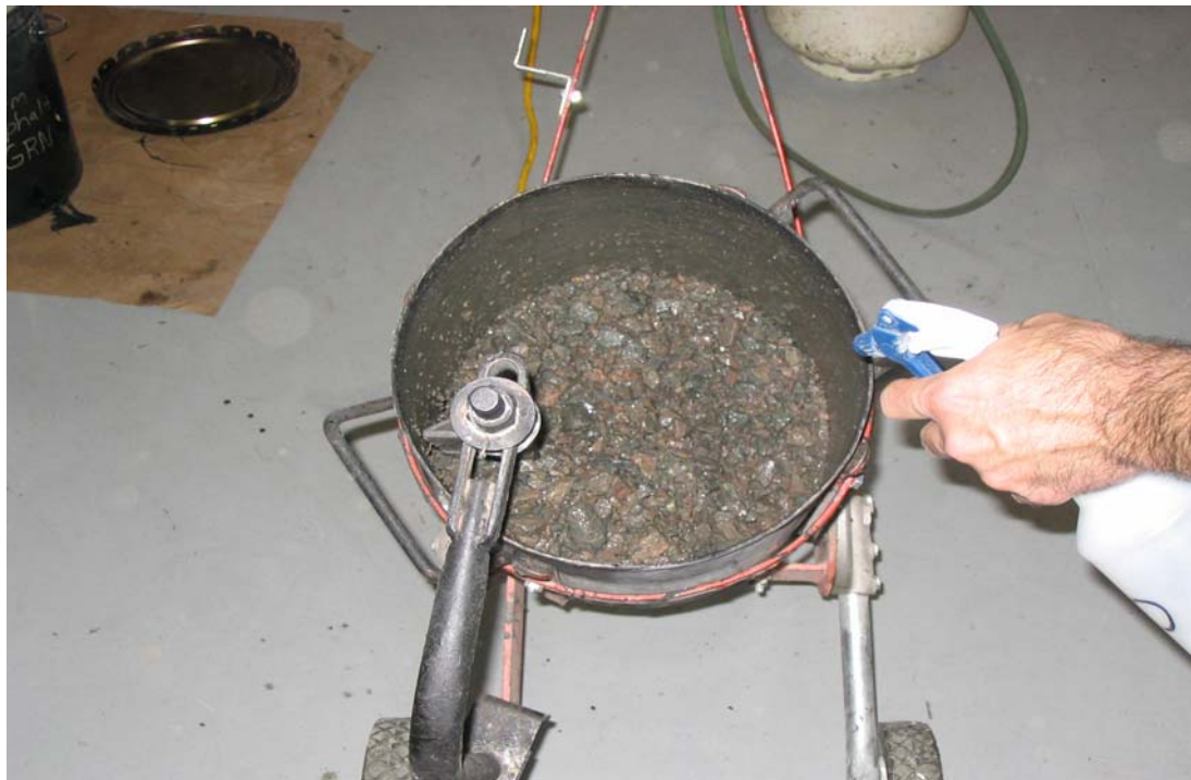
Figure 3. Introduction of Moisture to Aggregate for TSR Samples.
