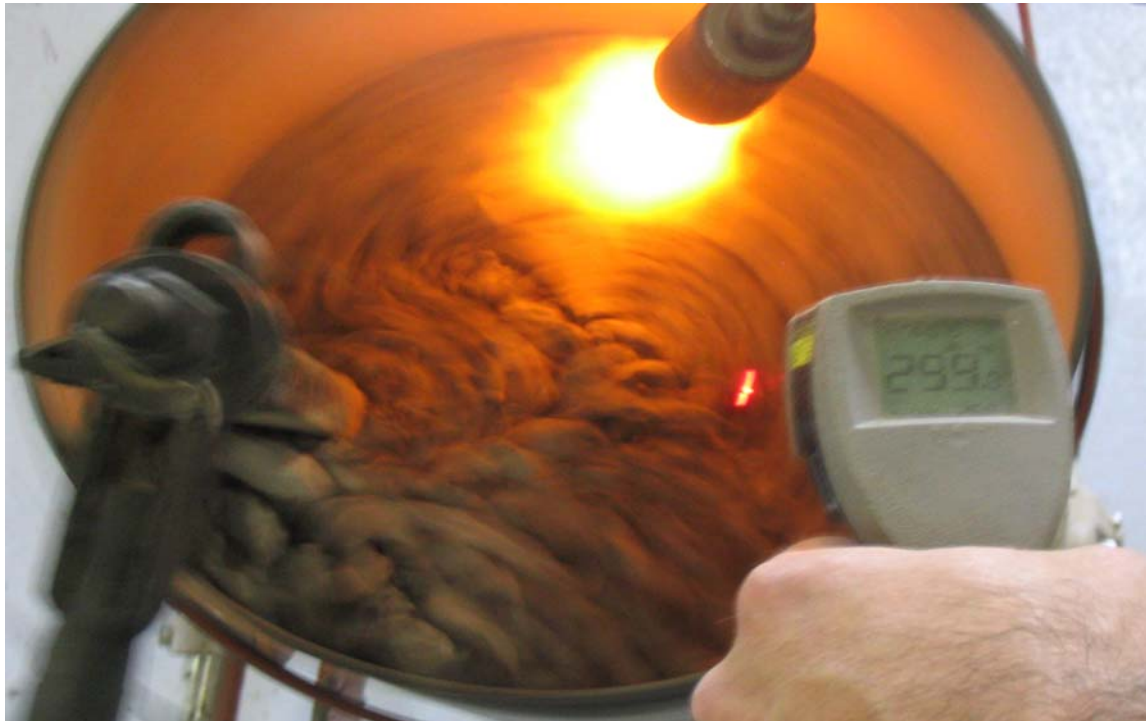
Figure 4. Heating of Wet Aggregate to Mixing Temperature.
