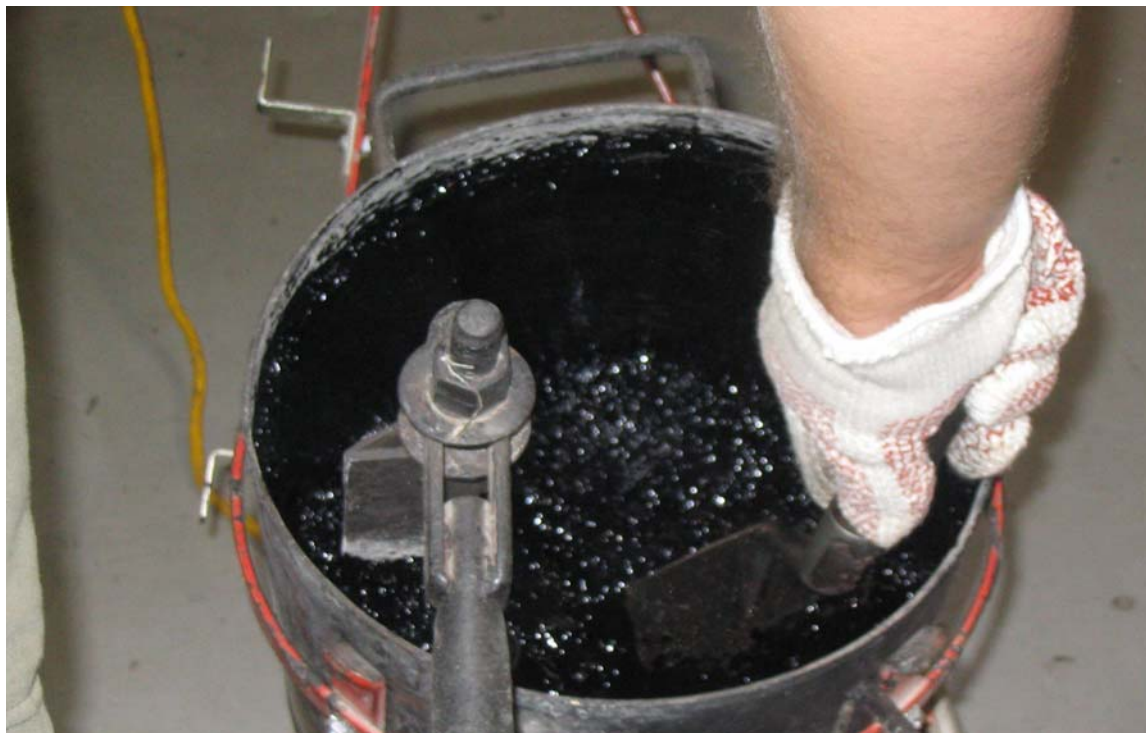
Figure 5. Warm Mix Asphalt in Bucket Mixer.
